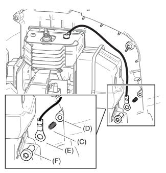
2. Insert compression spring V450-002470 (C) into hole (D) of fan case.
