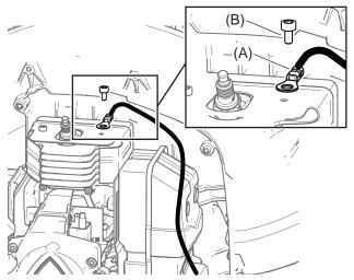
1. Tighten terminal (A) of lead V805-000240 to cylinder cover on exhaust side with bolt (B).
