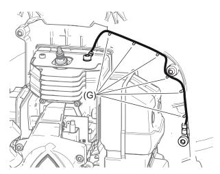
4. Route lead V805-000240 between 6 posts (G) and wall on fan case.
