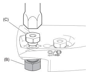
4. Install new collar nut (C) on the installer (B) and tigheten the nut (C) with a wrench until it bottoms.
