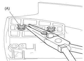
1. Remove remained collar (A) from the sprocket guard with longnose pliers.
