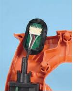
1. Connect power switch (A) and 6-pole terminal (G) of wire harness.
