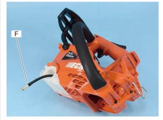
4. Pull out oil strainer (F) from oil tank.
