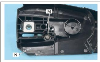
1. Place bevel gear (M) on sprocket guard (N).
