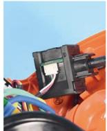
2. Connect variable speed switch (B) and 4-pole terminal (H) of wire harness.
