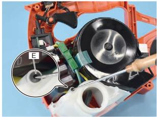
4. Put pointed tool into oil tank vent (E) and pull out the vent (E) while pressing the tool against the vent (E).
