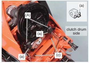
2. Install rib (a) of each cushion (A) in engine cover hole (c).
