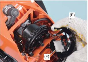
4. Assemble big air duct (E) with small air duct (F). Then tighten 2 torx bolts.
