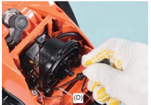
3. Use flat head screwdriver (D) when it is difficult to install rib (a) of each cushion.
