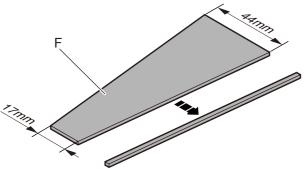
3. To seal exhaust port of cylinder, cut pressure rubber plug 91041 (F) off as shown.
