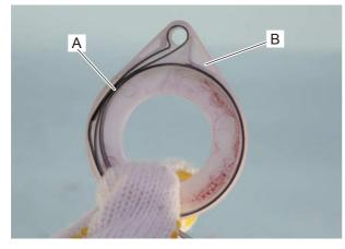
1. If rewind spring (A) is unwound from rewind spring case (B), wind the spring (A) inside case (B) as shown.
