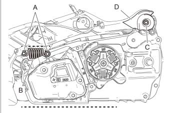
15. Install spring (B) and tighten two bolts (A).
