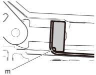
10. Push compression spring (N) with driver or other suitable tool and install compression spring (N) in sprocket guard as shown.
