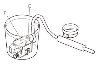
**NOTE:** To perform this test, carburetor interior should be wet with fuel. If dry, a little leakage may occur.
