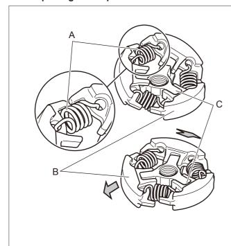
1. Install clutch springs (A) to clutch shoes (B).
