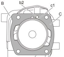
3. Set new cylinder gasket (C) on cylinder (B), as notch (c1) of gasket (C) aligns pulse hole (b2).
