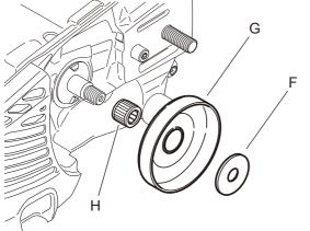
6. Remove clutch plate (F), clutch drum (G), needle bearing (H).
