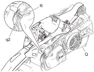
**NOTE:** Make sure boss (R) of rear handle insert to hole (q2) of enigne cover (Q) as shown.
