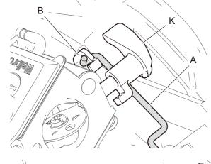
1. Connect throttle rod (A) to throttole lever (B), passing under choke knob (K) as shown.
