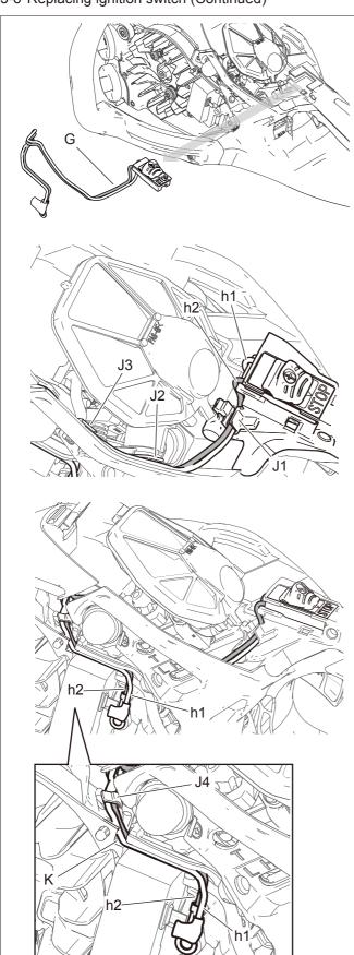
4. Remove ignition switch (G) from the unit as shown.
