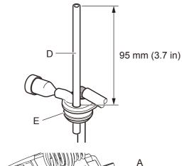
16. Reinstall fuel return line (D) through grommet (E) as shown.
