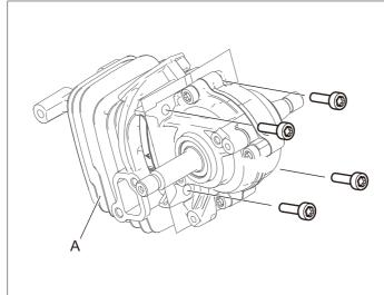
1. Remove four bolts securing cylinder (A) and remove cylinder (A).
