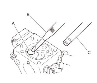
If engine does not run smoothly even after readjusting carburetor and inspecting carburetor parts, inspect low speed ports on carburetor as follows:
