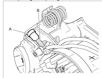
**NOTE:** Tank vent prevents a vacuum from forming in fuel tank when fuel in fuel tank is being consumed. When pressure in fuel tank becomes too high, tank vent releases the pressure.
