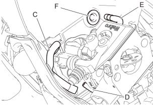
2. Connect purge line (C) and joint (D) of carburetor and install fuel inlet (E) of carburetor to fuel line (F).
