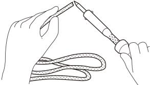
3. When installing a new starter rope, singe both ends of the rope to prevent fraying.
