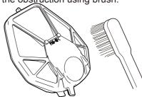
4. If heavily blocked with dirt or dust, clean the air filter with compressed air or wash away with non-inflammable solvent/detergent.
