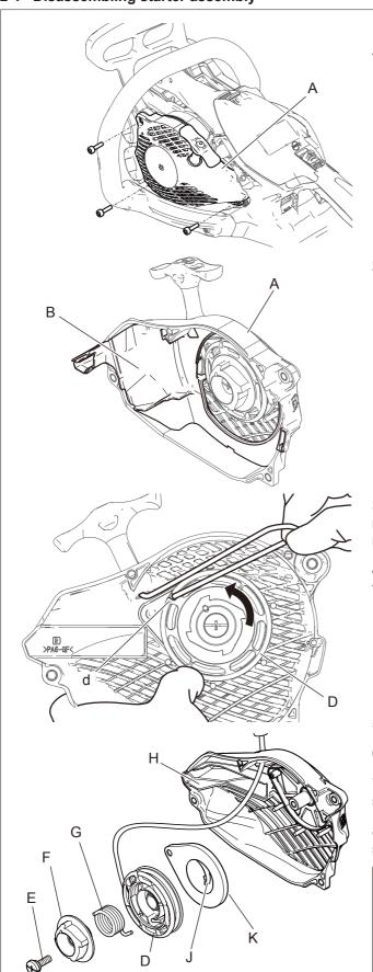
1. Remove three bolts and starter assembly (A) from the unit.
