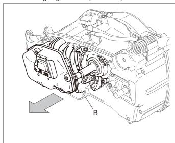
4. Pull out engine block (B) as shown.
