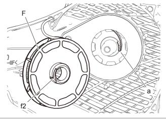
5. Assemble rope reel (F) engaging hook (f2) with hook (a) of rewind spring.
