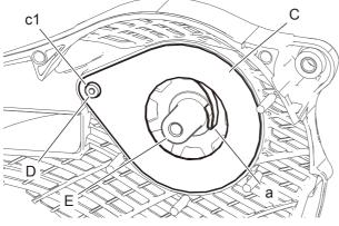
2. Carefully install rewind spring case assembly (C) on starter case, matching hole (c1) with post (D). Hook (a) of rewind spring should contact with post (E) of starter case.
