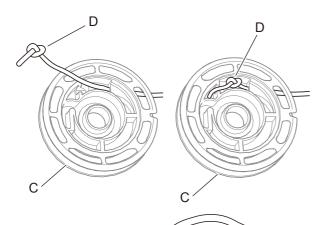
4. Make a knot (D) at end of starter rope and pass the rope through hole of rope reel (C), then press the knot (D) into recess as shown.
