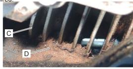
4. Remove ignition coil (E) if cylinder fins are hard to clean. Inspect the clearance of cylinder fins and the clearance between cylinder and engine cover. Clean the clearance using wooden stick or plastic stick or compressed air if dust is found.
