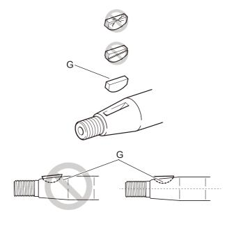
8. Inspect woodruff key (G) for damage or shearing. Replace as required.
