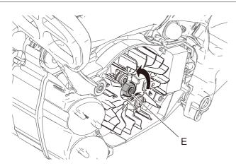
5. Remove nut (E) by rotating counterclockwise.
