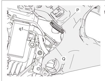
14. Install intake pipe (P) into groove (q1) of engine cover (Q) and then assemble rear handle.
