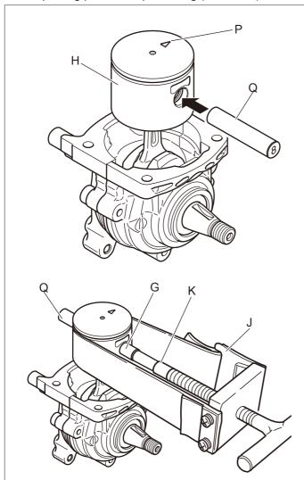
**NOTE:** Make sure to place piston with piston arrow mark (P) pointing as shown.
