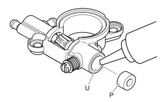
30. Apply grease in plunger hole (U). Tap plug (P) into hole (U) with plastic mallet until plug (P) is flush with end face of oiler body.
