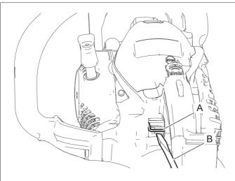
1. Unhook ring (A) with screwdriver (B) or equivalent and open cap cover (C).
