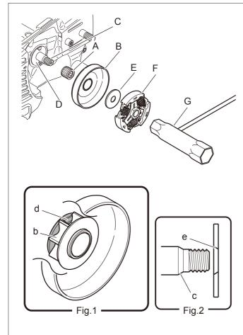
1. Apply lithium-based grease to needle bearing (A) and install needle bearing (A) and clutch drum (B) on crankshaft (C).
