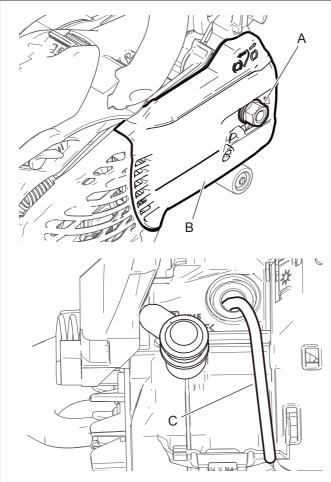
1. Loosen nut (A) and remove sprocket guard (B).
