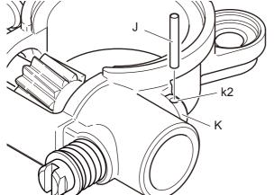
28. Press adjuster needle (K) to the bottom, orienting the flat surface (k1) as shown. This position indicates maximum discharge volume of chain oil.
