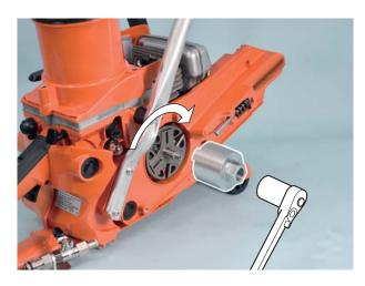
1. Install piston stopper X644-000020 in spark plug hole to stop crankshaft rotation.
