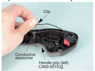
Install clip on control cable assembly V043-001180 or V043-001190 to the rib made of conductive elastomer.
