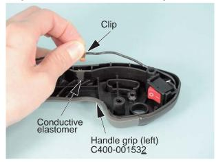
Install clip on control cable assembly V043-001170 to the rib made of conductive elastomer.
